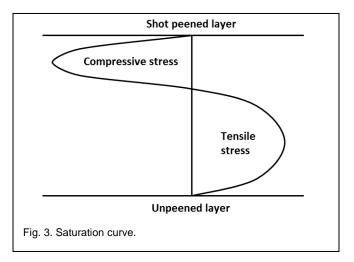
If a thin material is peened on one side a curve will develop in it and the shot peened side will be convex. This formed the basis of the standard Almen strip which is used for the measurement of the shot peening intensity and the control of the process. The Almen strip test method is, so far, the only available non-destructive method for determining the peening intensity.
